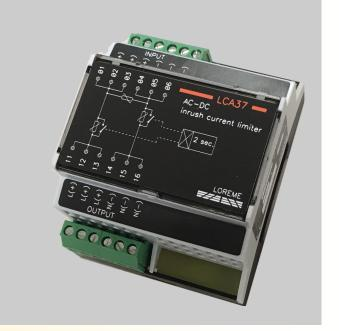
The LCA37 is a active inrush current limiter with a temporized bypass relay ensuring a more efficiency operation compare to a NTC. It cut-off the current peak in the load at the installations start-up and does not dissipate power when operating.
